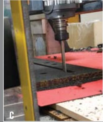
Your layout is then transferred to your choice of foam to be cut using either (A) Water Jet Technology, (B) Die Cut Technology or (C) CNC Router Technology.
